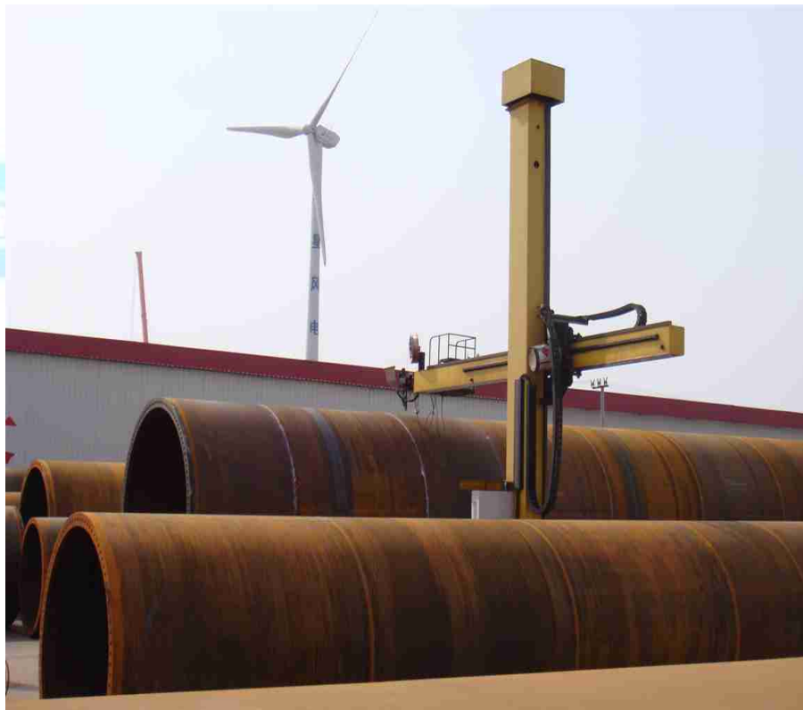
Welding manipulator used in wind power industry
