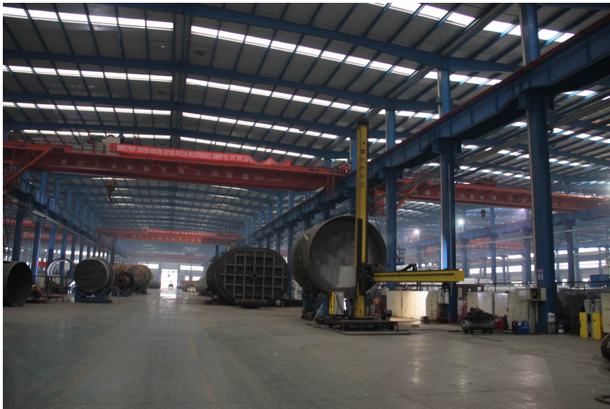
Welding manipulator used in chemical industry
